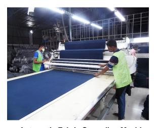
Automatic Fabric Spreading Machine With Vacuum Table
